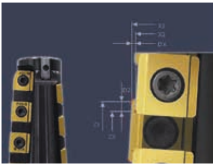
Measuring lateral and transverse dimensions of cutting edge overlap (Measuring program 736)
